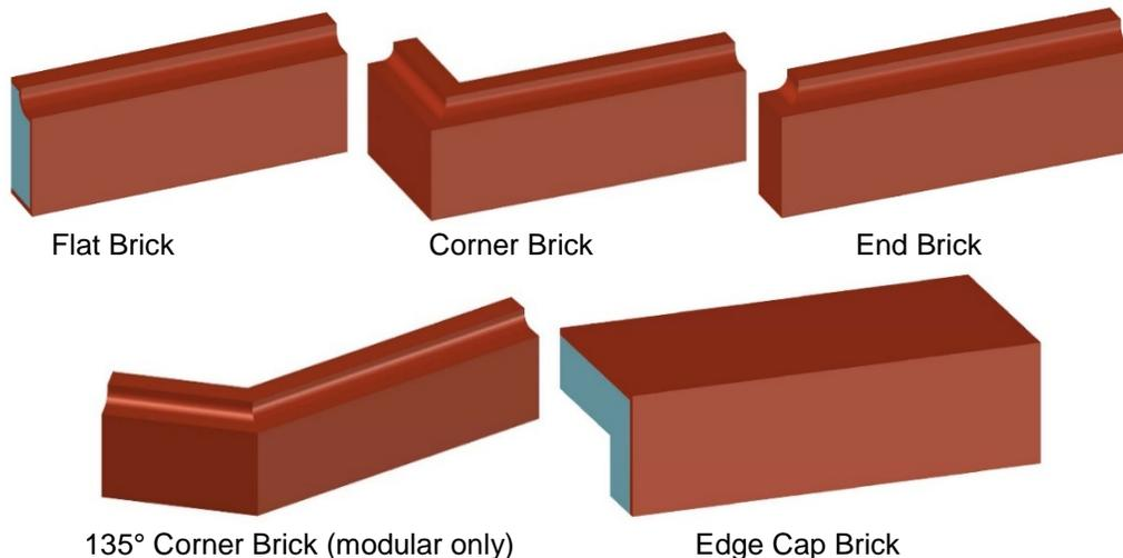
**Figure 1:** Flat Brick, Corner Brick, End Brick; 135° Corner Brick and Edge Cap Brick Configuration
