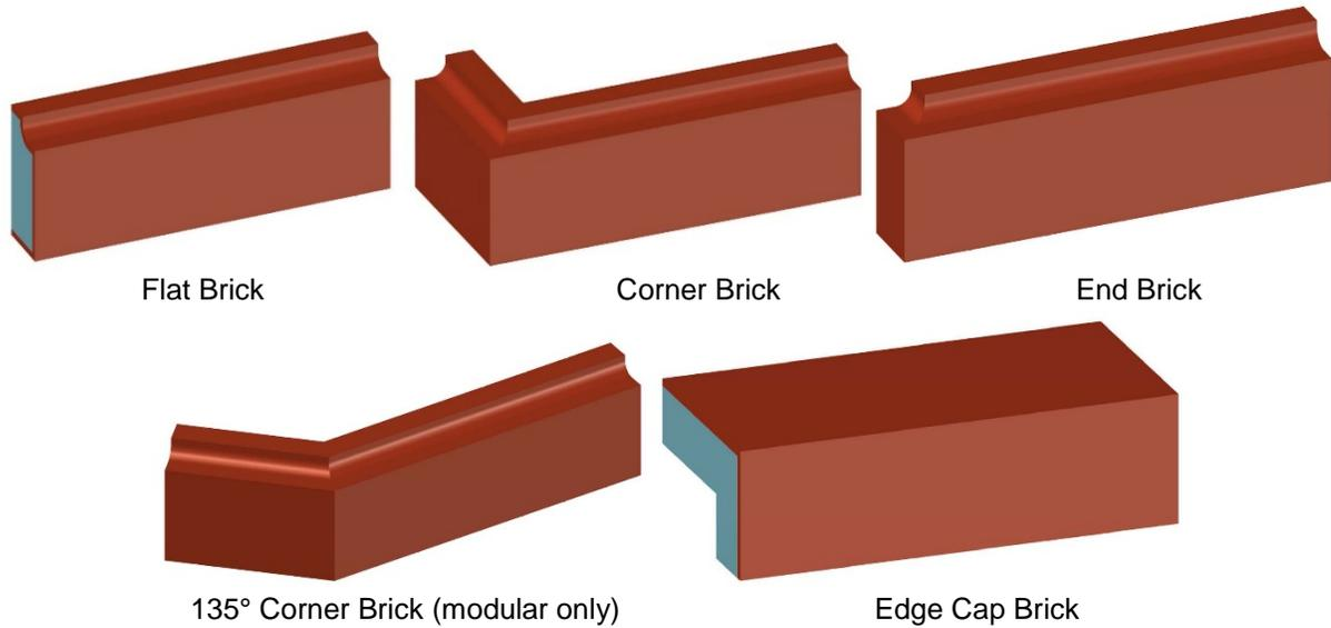
**Figure 2:** Flat Brick, Corner Brick, End Brick; 135° Corner Brick, and Edge Cap Brick Configurations
