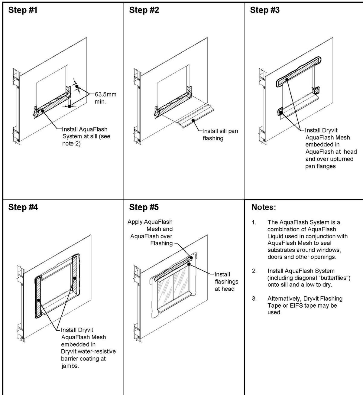
Figure 3: Rough opening and sill preparation – AquaFlash System
